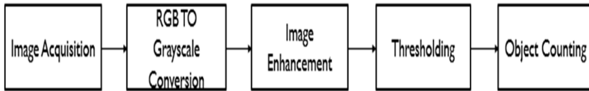
Fig. 3: Block Diagram Representation of Thresholding Method
