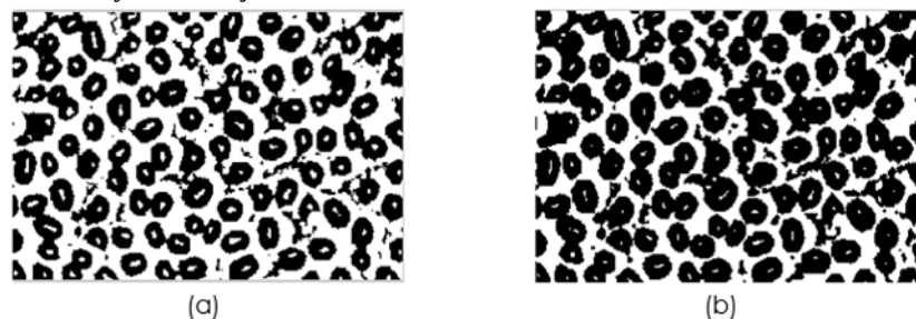
Fig. 6: Simulation Results for Dilation (A) Image after Thresholding (B) Image after Applying Dilation
