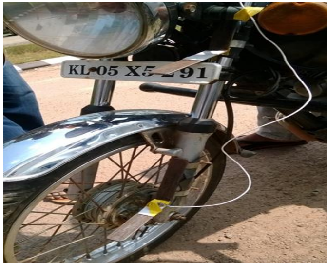
Fig. 1: Fixtures for Accelerometer
