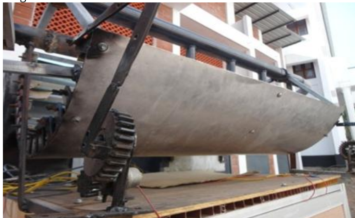
Fig. 2: Solar Parabolic concentrator
