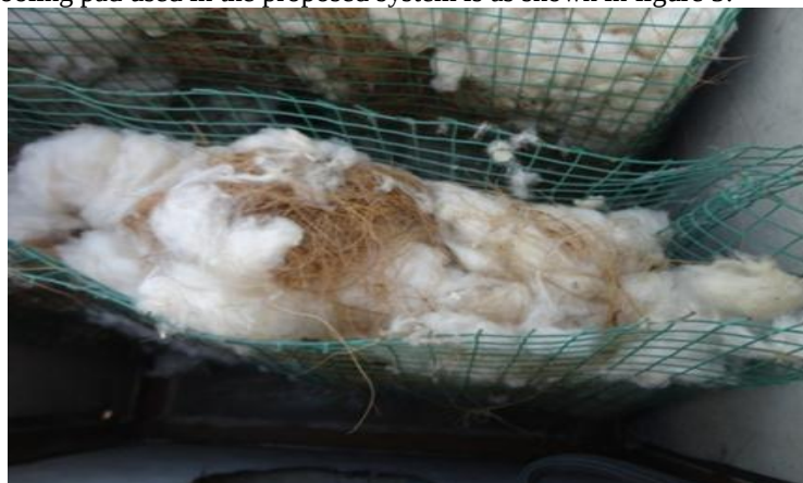
Fig. 5: Cooling pad used in the fabricated system
