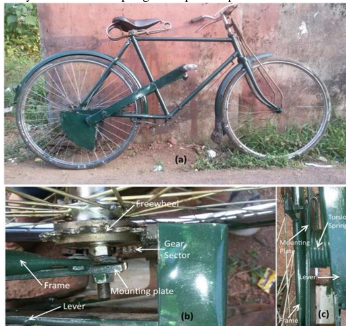
Fig. 1: (a) Lever Driven Bicycle. (b), (c) Parts of Lever Driven Bicycle.
