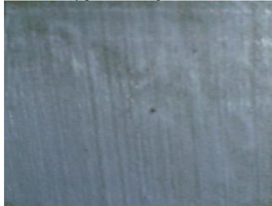
Fig. 11: Pin holes on the surface of a billet observed by magnifying glass
