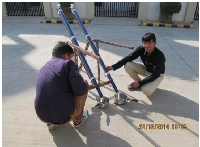
Fig. 2: Tilting arrangement for molten wax
