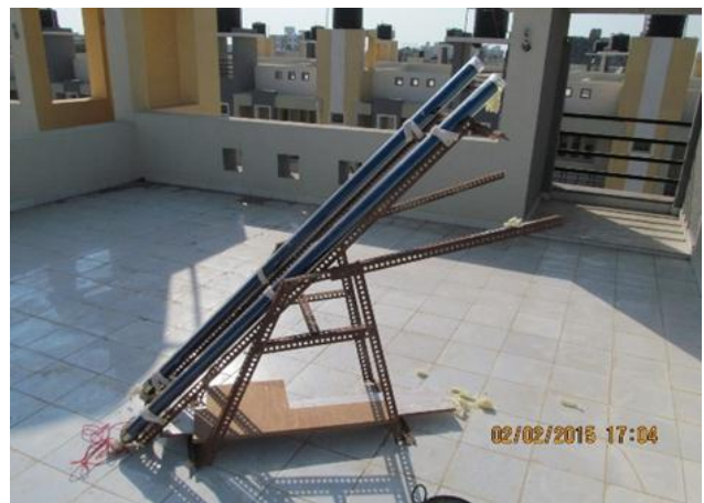
Fig. 4: Heating paraffin wax in ETC
