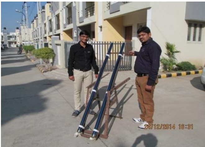
Fig. 1: Solar evacuated tube collector (ETC) set up for paraffin wax Melting
