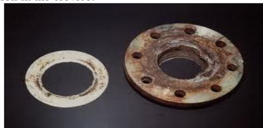
Fig. 7: Crevice corrosion
