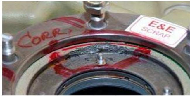
Fig. 2: Corrosion damage in magnesium alloy castings used in rotor
