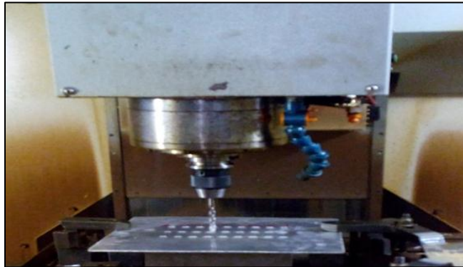
Fig. 1: Drilling on GFRP Sheet
