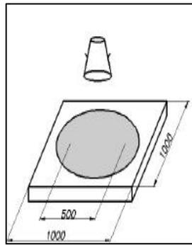
Fig. 1: Slump Flow Test
