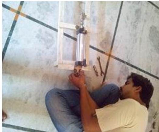
Fig. 5: Fitting Pump on Base
