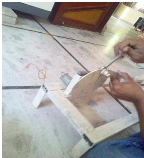
Fig. 6: Fitting Connecting Rod with Disc
