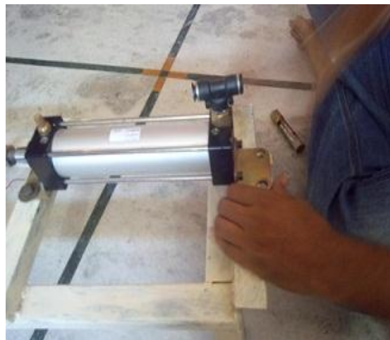
Fig. 8: Attaching Tee with Pump
