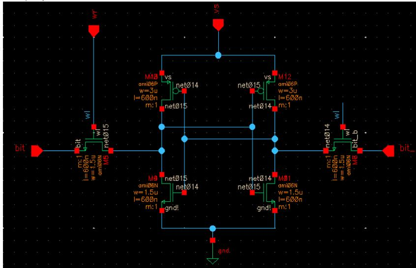
Fig. 3: 6T-SRAM Cell Architecture
