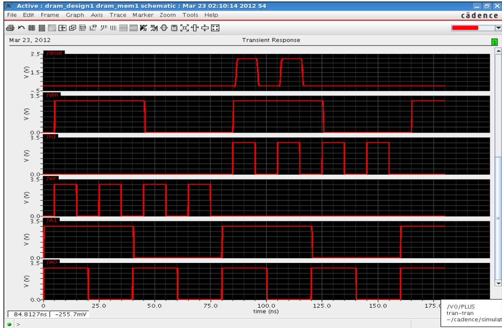
Fig. 8: Results of 3T1D DRAM for 0.60um ami
