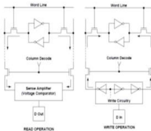
Fig. 4: SRAM Cell Read/Write Operation
