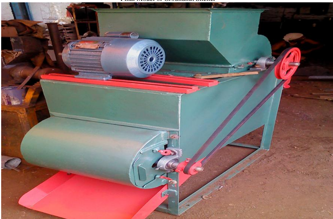
Final Model of Groundnut Sheller
