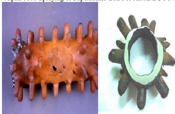
Fig. 4: Failure of In-Bed Evaporator Tube
