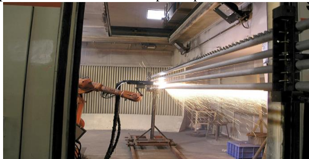
Fig. 3: Alpha 1800 Spraying of Superheater Coil For An AFBC Power Plant
