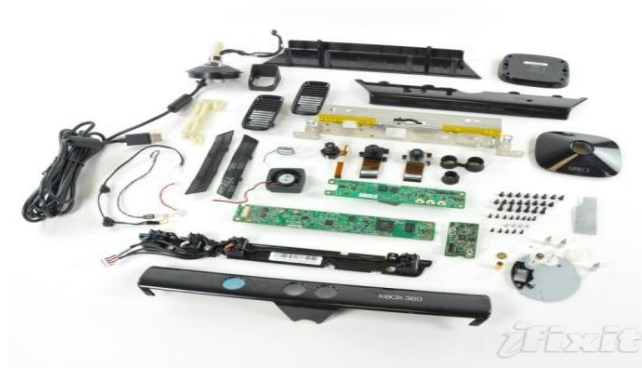
Fig. 1: Hardware Component of The Kinect Device
