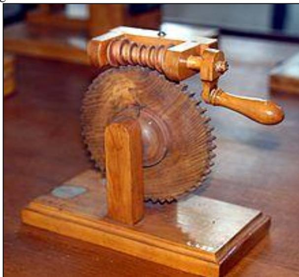
Fig.1: Worm and Worm Gear
