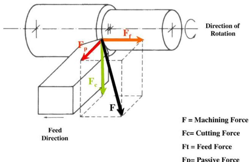
Fig. 1: Schematic Draw of The Machining Forces Components In A Turning Operation
