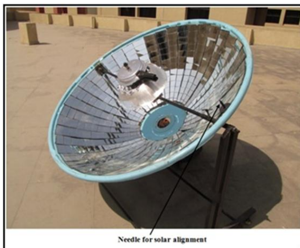
Fig. 5: Needle indicator for solar alignment of commercial cooker
