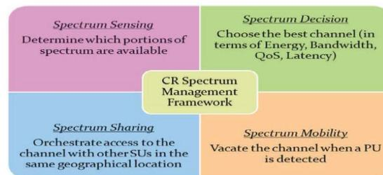
Fig. 4: functions of cognitive radio (spectrum management)
