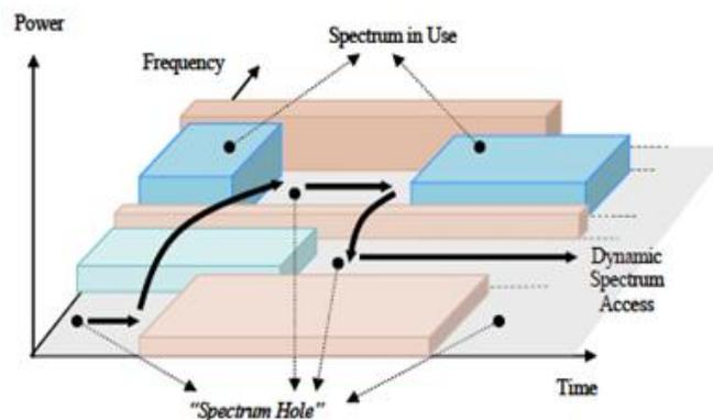
Fig. 2: spectrum hole and dynamic spectrum access
