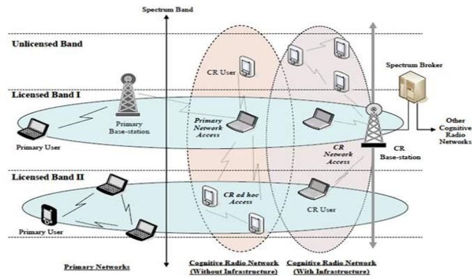
Fig. 3: cognitive radio network architecture
