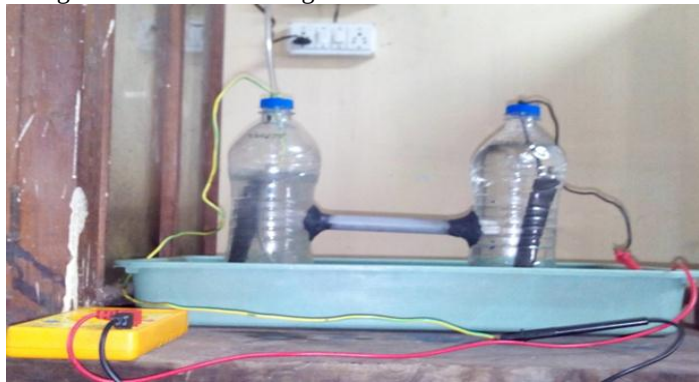
Fig. 1: Microbial Fuel Cell for the treatment of Waste water
