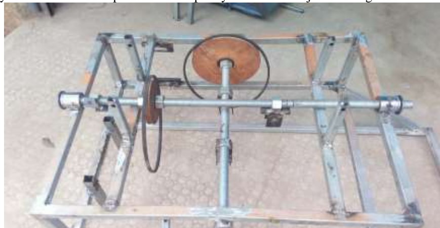
Fig. 8: power screw mechanism and its supports.
