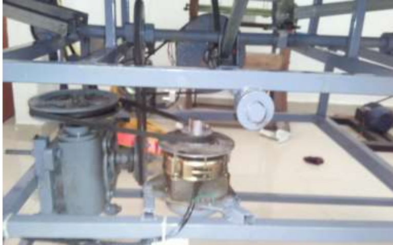
Fig. 9: The power screw is driven using a single phase induction motor.
