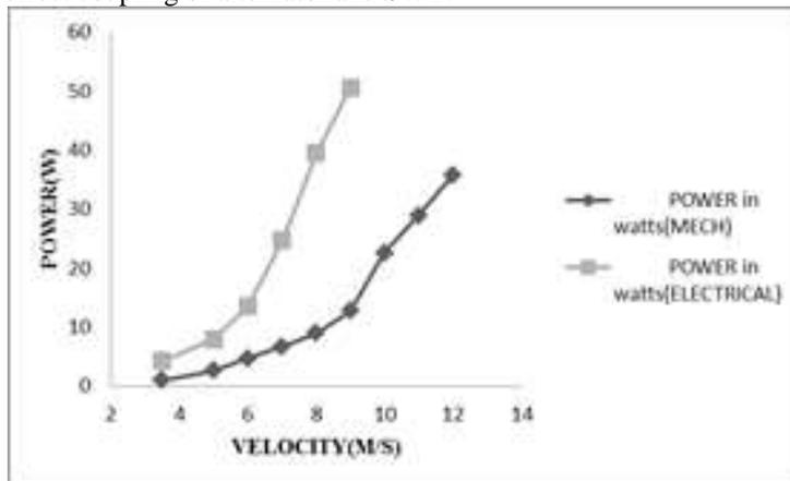
Fig. 4: velocity vs power (without gear)
