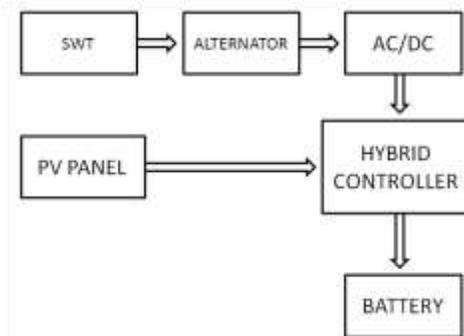
Fig. 1: Block Diagram Of Hybrid System
