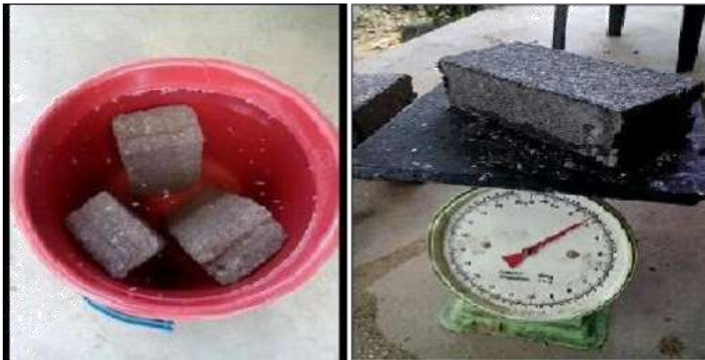
Fig. 6: Water Absorption test
