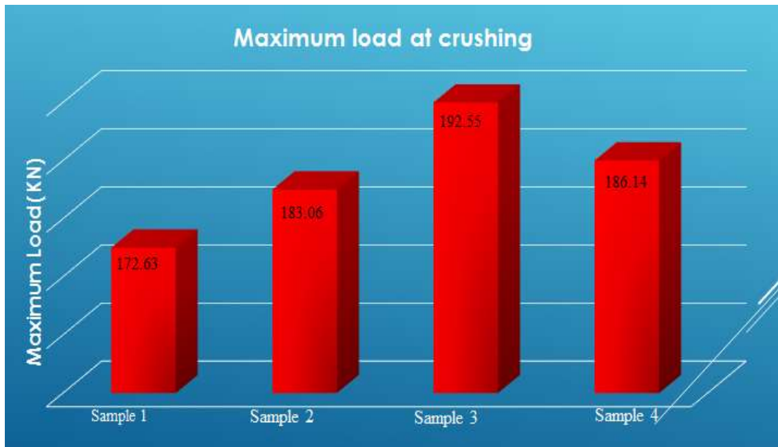
Fig. 7: Effect of different ratio of plastic waste on compression test
