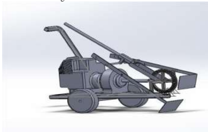
Fig. 3.1: Design model of soil scooping machine
