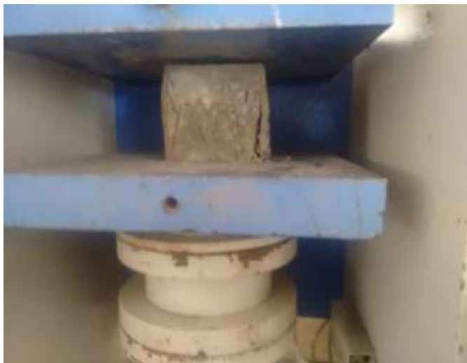
Fig. 4: Compressive strength test
