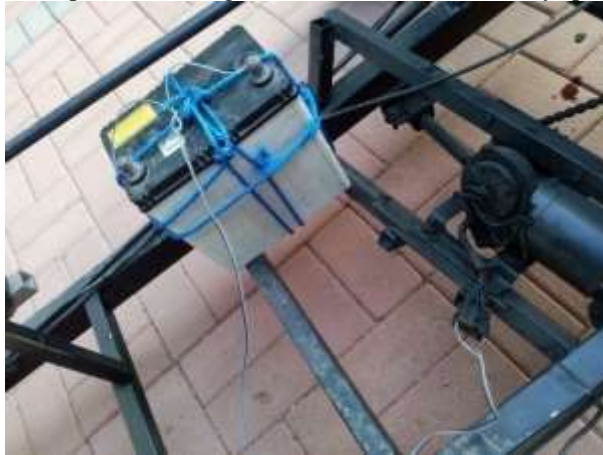
Fig. 4: DC motor and Battery
