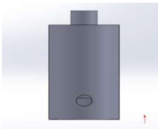
Fig. 5: Front view of gasifier unit
