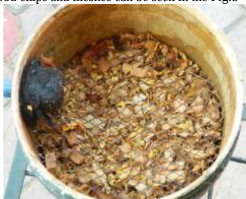
Fig. 8: Loosely packed wood chips in the particulate filter
