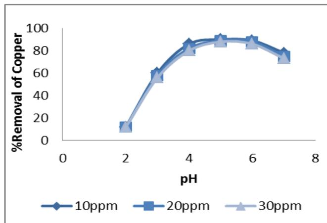
Fig. 1.8: Effect of pH on %removal of copper ion by tea waste adsorbent.
