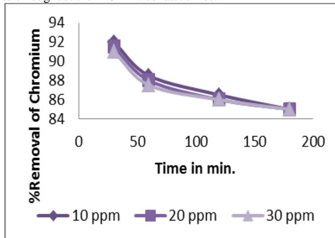
Fig. 1.5: Effect of contact time of %removal of chromium ion by tea waste adsorbent.
