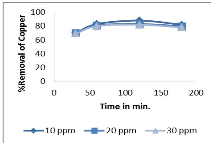
Fig. 1.6: Effect of contact time of %removal of copper ion by tea waste adsorbent.
