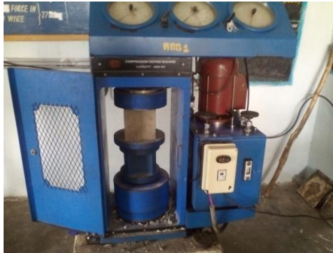
Fig 2: Testing of geopolymer concrete cubes.
