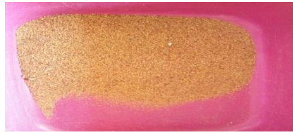
Fig. 3.2: After Wet Sieve Analysis Of Laterite Soil
