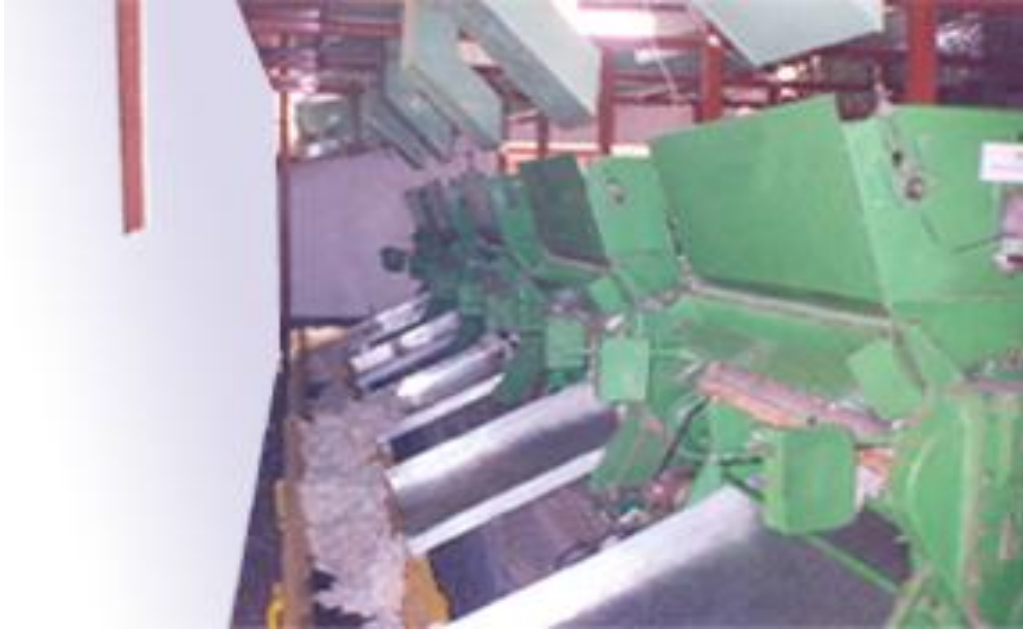
Fig. 1: Belt type lint conveying system Working Principle
