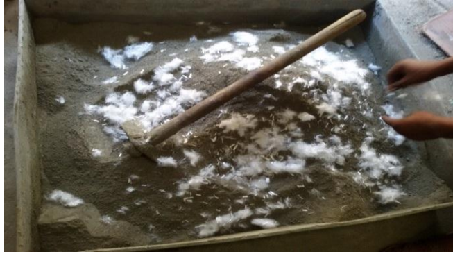
Fig. 1: mixing of polypropylene fibres in mortar
