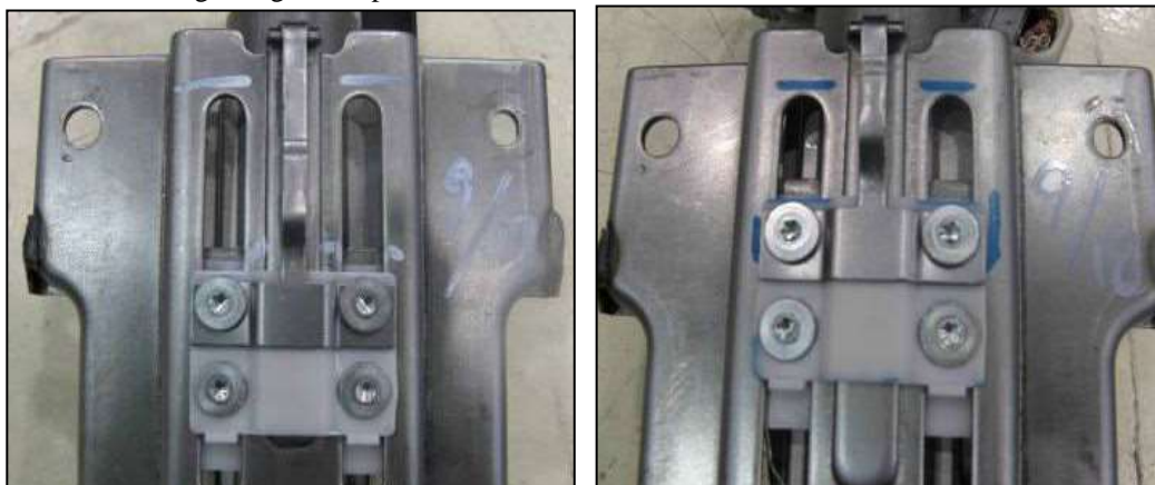
Fig. 4: Column Collapse distribution of sled test
