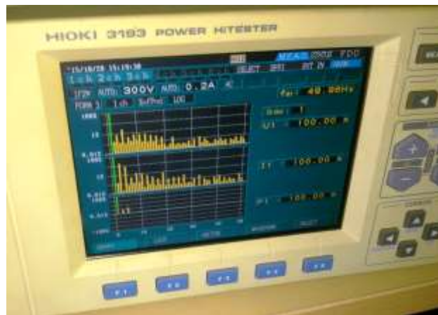
Fig. 12: value of U, I, P display by analyzer using of 4700 \mu f capacitor
