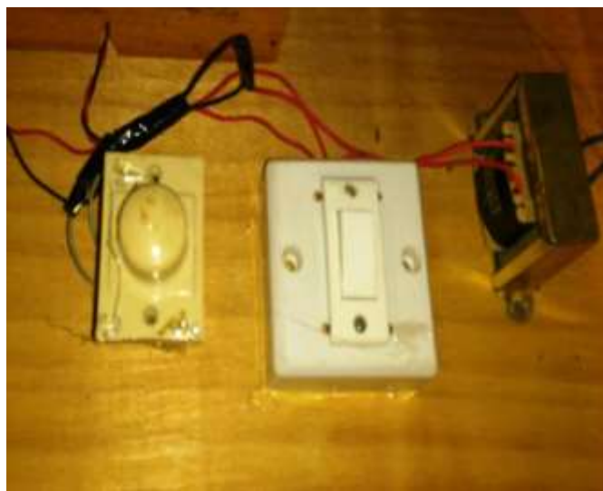
Fig. 1: Power supply with Regulator
