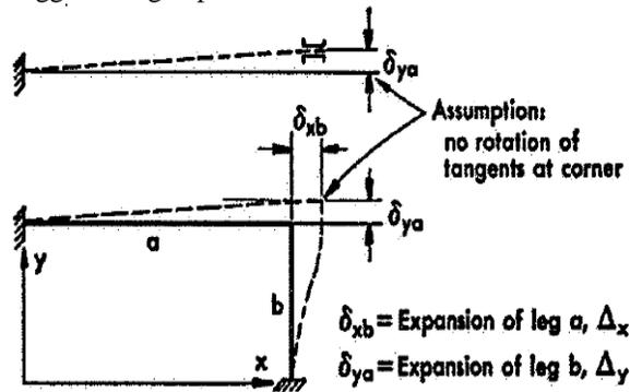
The individual legs absorb the following portion of the thermal expansion. ( Y-direction):
