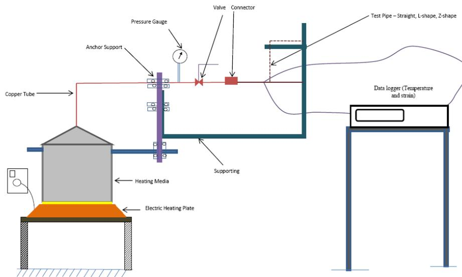
Fig. 3: Experimentation set-up
