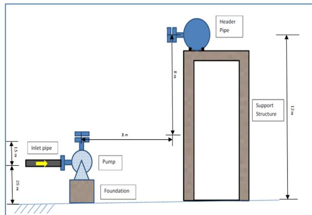
Fig. 2: Pump and Piping connection required
