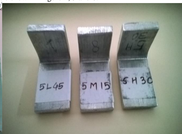
Fig. 4: Specimen after L bending (5mm)
