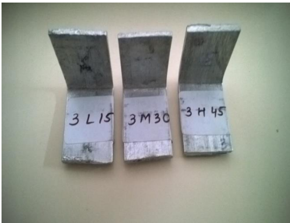
Fig. 5: Specimen after L bending (3mm)
