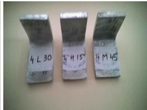
Fig. 6: Specimen after L bending (4mm)
