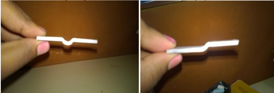
Fig. 9: Specimen after reverse bending and half straightening
