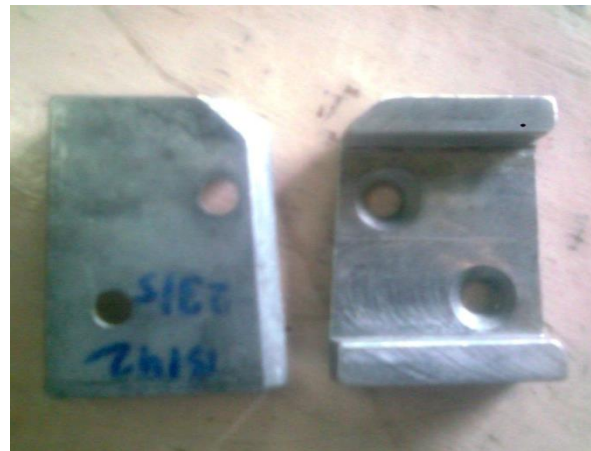
Fig. 4: Finished product for Micro hardness, Surface roughness and Microstructure [After machining Dovetail]
