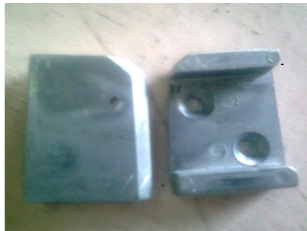
Fig. 3: Synthesis of Al alloy with SiC composite using Stir casting route [As cast Dovetail]
