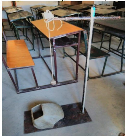
Fig. 12: Drop Test On The Scoop
