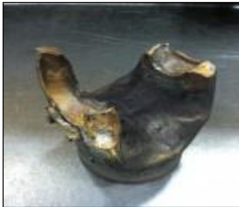
Fig. 6: Weld Yoke Failure (3)
