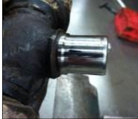
Fig. 2: Universal Joint Brinelling (3)
