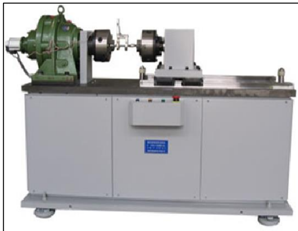
Fig. 8: Torque test set up
