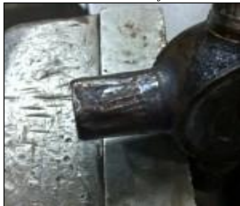
Fig. 4: Burned U Joint Trunnion (3)
