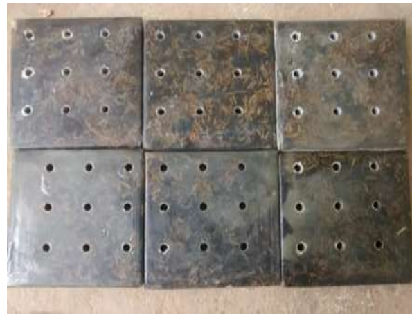
Fig. 2: Drilled Composite sample I II II (1st row without coolant 2nd row with coolant)
