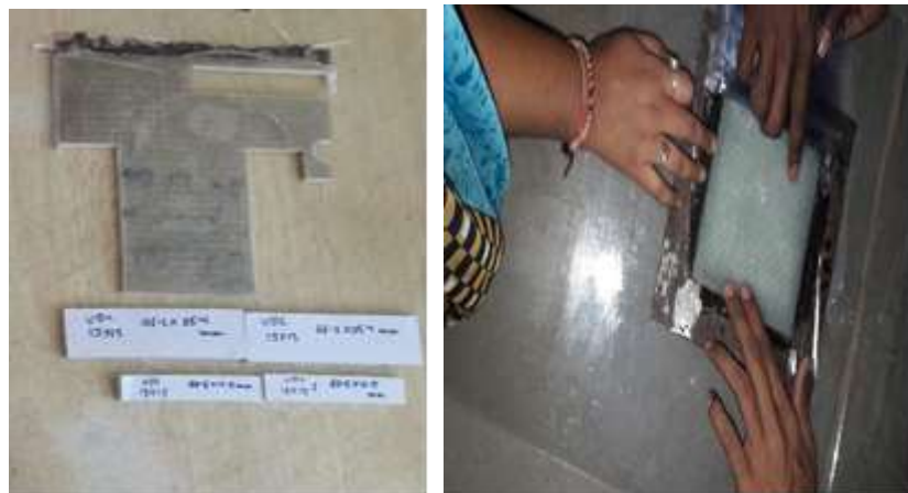
Fig. 2: Uni-directional and Bi-directional Glass fiber composite
