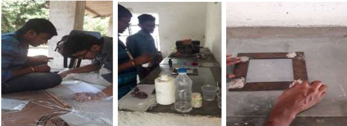
Fig. 1: Cutting of glass fiber and hand lay technique set up
