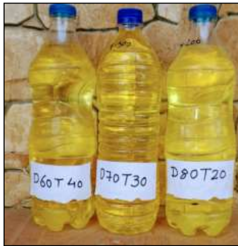
Fig. 2: Blend preparation of Diesel and Turpentine
