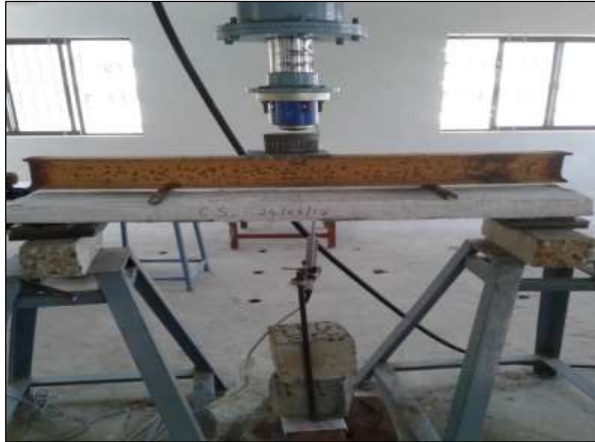
Fig. 5: Loading setup of slab specimen.
