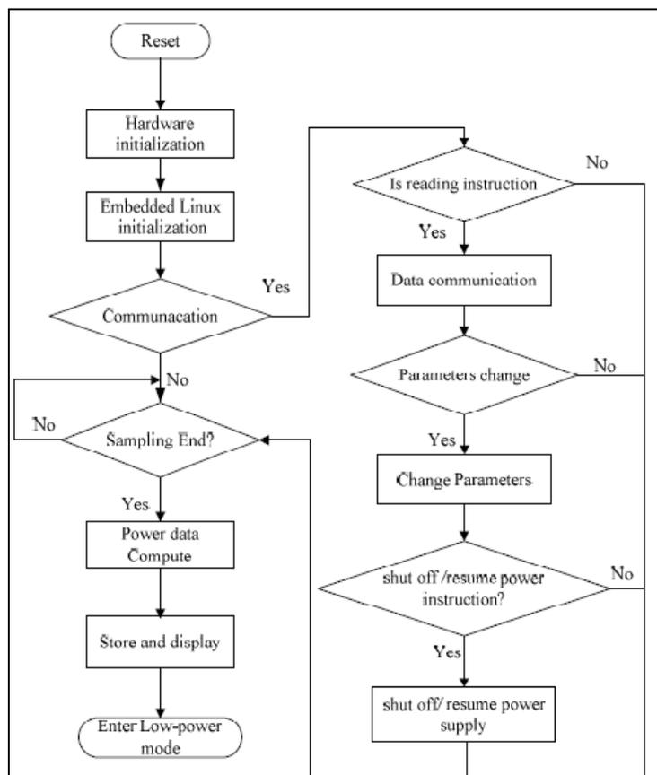
Fig. 3: The PMWCM system software flow chart
