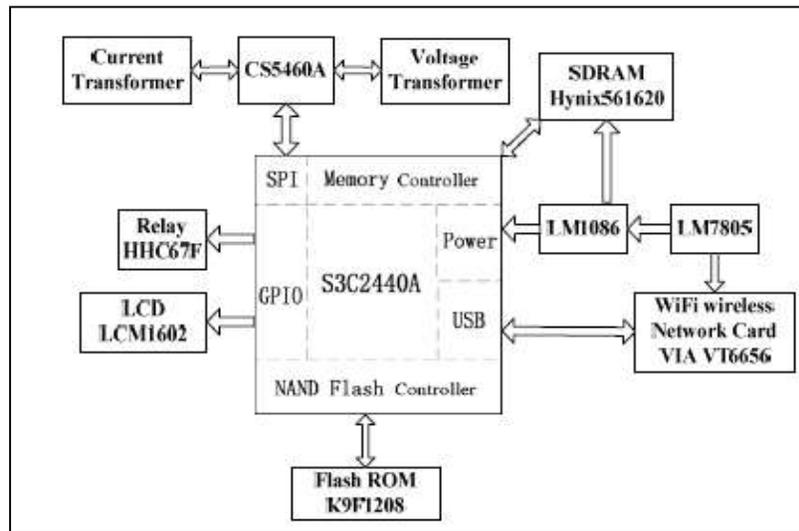
Fig. 2: The Hardware System of PMWCM
