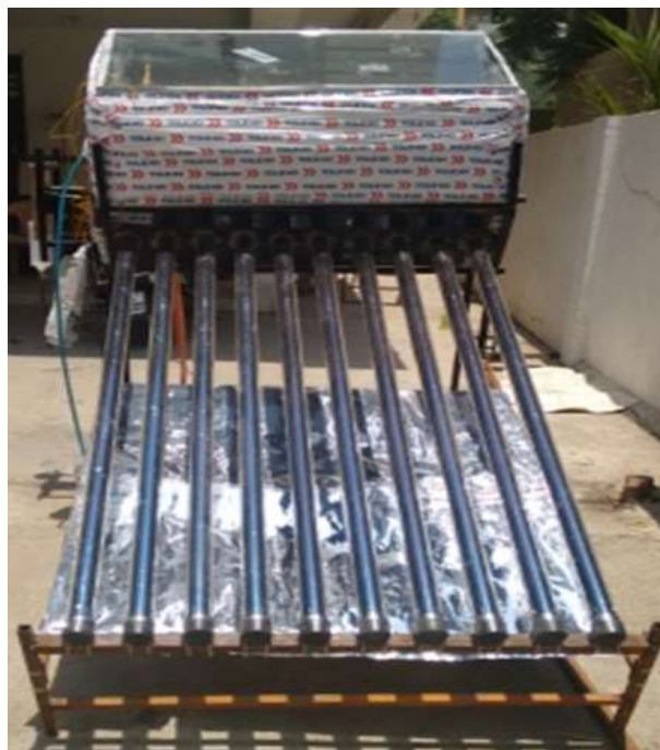
Fig. 2: Pictorial view of double basin solar still augmented with evacuated tubes
