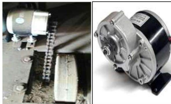
Fig. 5: DC Gear Motor Arrangement
