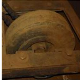
Fig. 12: Rubber driving wheel
