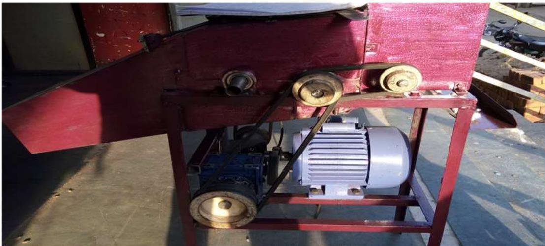
Fig. 2: Fabrication of Mini Cotton Ginning Machine
