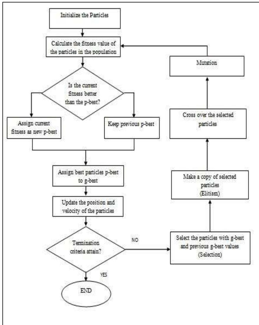
Fig. 5: Flowchart of Hybrid PSO-GA Algorithm
