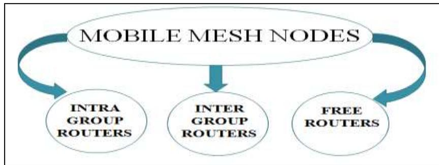
Fig. 1: classification of mobile mesh nodes
