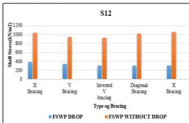
Fig. 13: Shell stresses v/s type of bracing for S12
