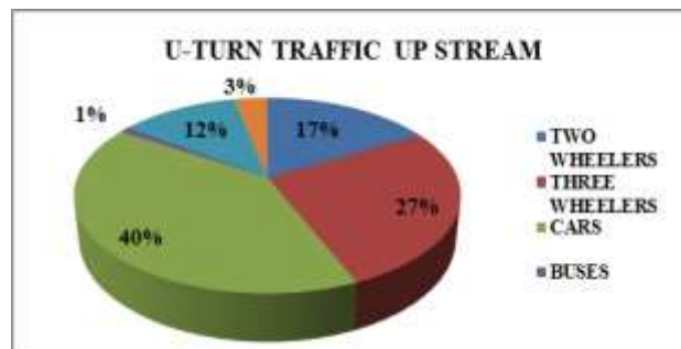
Fig. 3: Traffic Composition of U-turn traffic on Upstream direction
