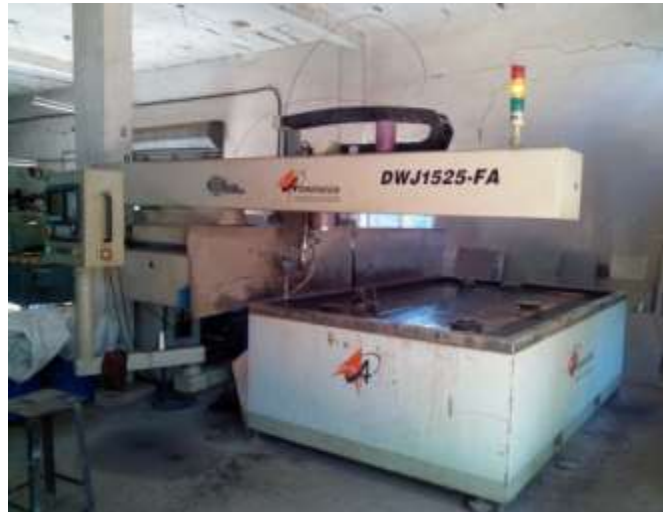
Fig. 1: Setup of abrasive water jet machine
